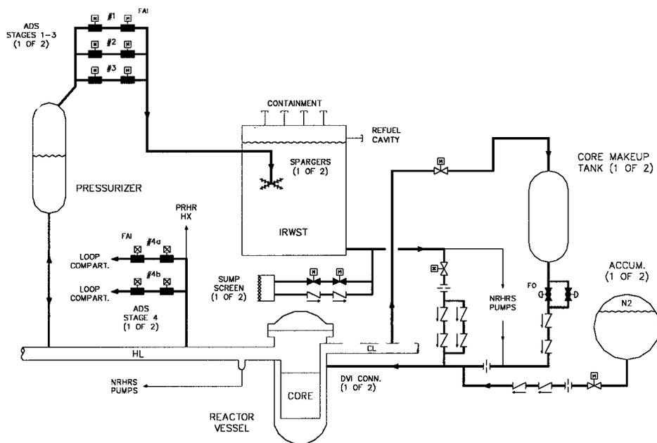
Figure 5 AP1000 Passive core cooling system
