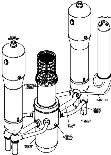
Figure 1 Isometric view of AP1000 NSSS
